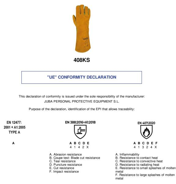
In accordance with EU Regulation 2016/425 and based on applying the EN 388:16+A1:18, EN 407:20, EN 12477:01+A1:05 and EN ISO 21420:20 standards, as PPE in Category II, identical to Certificate UE type no. C-01822-2022-1, issued by the notified body no. 0162 -LEITAT - C/ de la Innovació, 2, 08225 Terrasa, Barcelona.
